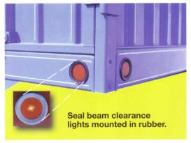
Heavy-duty rear corner post extends to bottom of platform and is integrated with rear rail to give strength to rear corner, with or without doors installed.
