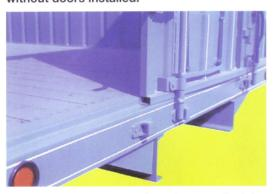
Rear rail is stepped to allow doors to fit tight. Door seal kit included.
